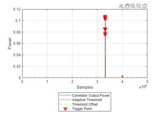
Inspect the trigger points by zooming in along the x-axis of the plot. For example, this figure shows a zoomed-in view of an OFDM packet with the trigger points on the correlation peaks.
